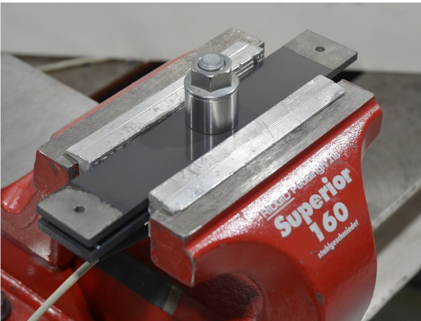
Figure 8 Assembly of test panels in a screw vice
